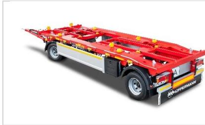
Flex-Carrier for the transport of roller and skip containers
