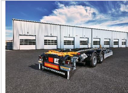
2-axle-central-axle-skid carrier for the transport of roll-off containers and swap bodies
